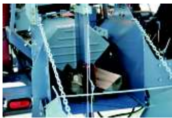
Two or Four Way Splitter options with 4" or 5" cylinder
