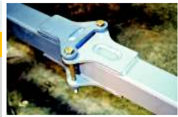
Fold-away hitch for an easy fit inside a garage, or for safety at the jobsite.
